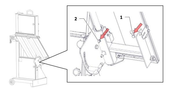
Lubrication points on the masonry band saw:
