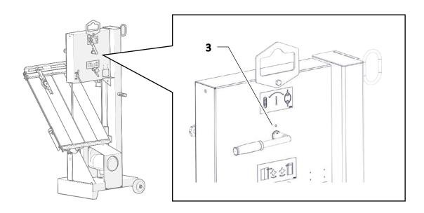
• Lubricate the automatic power chuck above the opening (Pos. 3) on the tensioning lever with a spray oil
